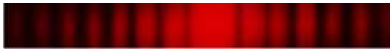
v) Single-slit diffraction of red light. Note the double width of the central maximum.
