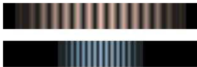
q) Double-slit diffraction patterns of long-wavelength red light (top) and short-wavelength blue light (bottom).
