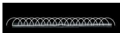
h / If it was by itself, each of the parts would spread out as a circular ripple.
